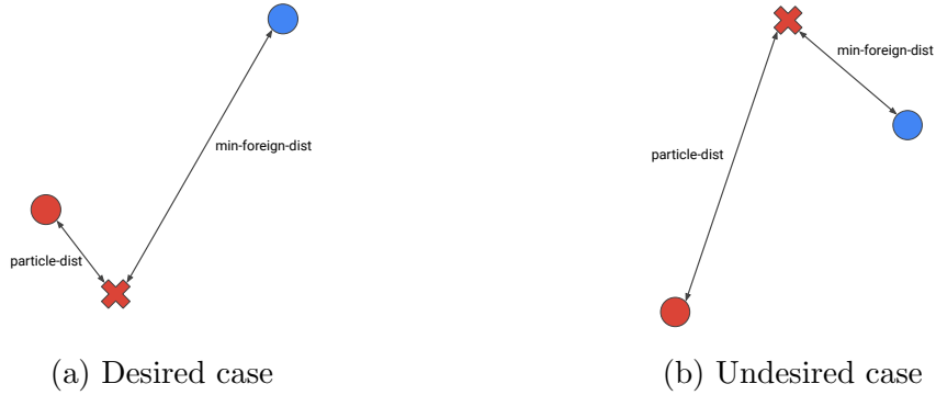
Figure 5-1: Visualization of prediction quality. Predictions are marked as crosses, hits as circles
